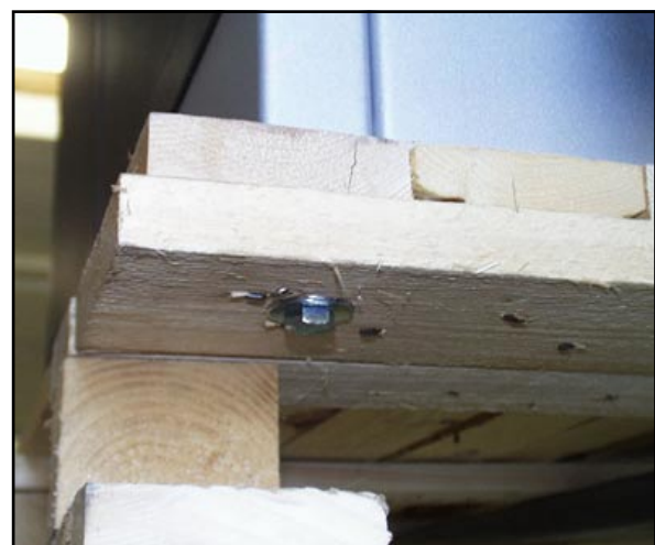
Fig. 3-D. Processor on pallet. Shipping Screws are holding it on.
